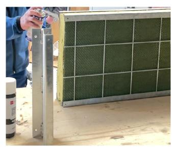
3. Use the repair spray to seal and protect the trimmed metal parts.
