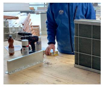
**2.** The adjustment kit/profile is used to establish a new mounting flange.
