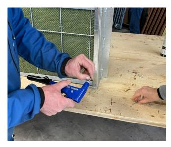
4. Place the mounting flange on the side of the module. Secure it with the supplied screws, or with pop rivets if available. The module is now ready for installation.
