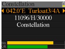
• 042.0°E Turksat3/4A: The current satellite. Press [ ◀ / ▶ ] to switch between satellites and press [OK] to enter satellite list to select satellite.
