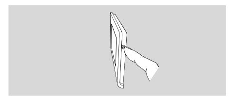
A **short press** (1 second) of the side button switches on the display and all connected N-BUS devices. A **long press** (5 seconds) of the side button switches off the display and all connected N-BUS devices.
