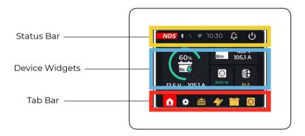
The tab bar shows the icons of the active devices connected to the N-BUS network, the setting icon (Settings) and the return button to the Home Screen are also shown.
