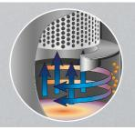
DV-Series compressors are fitted with an effective three-phase separation system. Most of the oil is separated under centrifugal force in the separator tank. Some of the oil is separated by gravitational force during movement of oil inside the separator.
