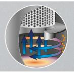
DV-Series compressors are fitted with an effective three-phase separation system. Most of the oil is separated under centrifugal force in the separator tank. Some of the oil is separated by gravitational force during movement of oil inside the separator.
