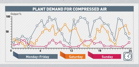
Conventional screw compressors are not able to switch between operating modes according to a plant's current demand for compressed air. Owing to constant switching between loading/unloading modes or the idle running of compressors, conventional screw compressors consume consistently large amounts of electrical energy when operating. The Comprag AV compressor series with frequency control has been created for economical compressor operation where there is varying demand.
