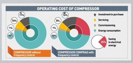
AV compressors are provided with a frequency converter for continuous control of compressor output according to the current demand for compressed air. They provide a plant with the necessary amount of compressed air at a given moment and at a constant set pressure, while consuming only as much electrical energy as there is demand for compressed air. This mode of operation conserves as much energy as possible.
