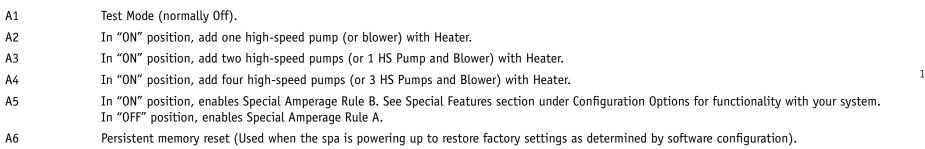
A2, A3, and A4 work in combination to determine the number of high-speed devices and blowers that can run before the heat is disabled. i.e. A2 and A3 in the ON position and A4 in the OFF position will allow the heater to operate with up to 3 high-speed pumps (or two HS Pumps and Blower) running at the same time. Heat is disabled when the fourth high-speed pump or blower is turned on.
