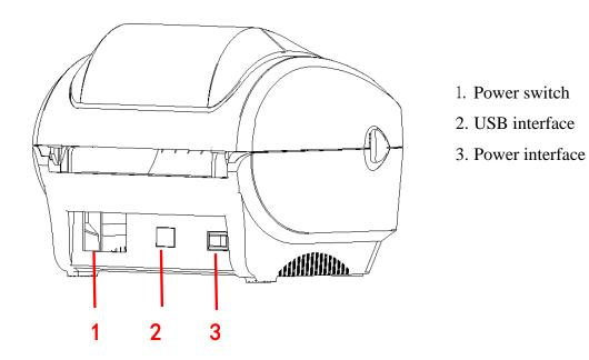
Note: The transmission interfaces of the printer in the picture will vary depending on the model of machine you purchase. For the actual transmission interface, please refer to the catalog specifications.
