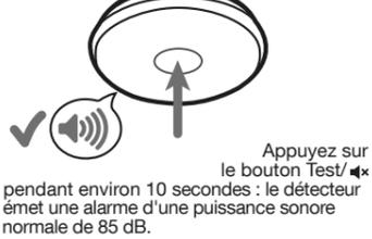
**LE DÉTECTEUR DOIT ÊTRE INSTALLÉ SUR SA PLATEFORME DE MONTAGE AFIN DE POUVOIR DÉCLANCHER UNE ALARME.**
