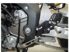
Mount a shifting lever according to photo 5.
