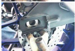
1. Remove rear axle lock nut & axle.
