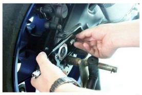
6. Assemble screws with chain adjusters in a proper way.
