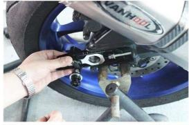
7. Install left & right side chain adjuster, tighten#2 original screws.
