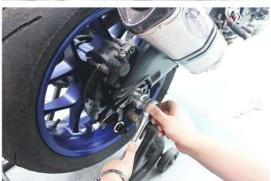
8. Reinstall rear axle & lock nut, adjust drive chain to factory specs with left & tight side chain adjuster knobs. Tighten and lock all bolts as shown. (Please lock & tighten axle lock nut and adjust the torque from 95N. M-110N.M).
