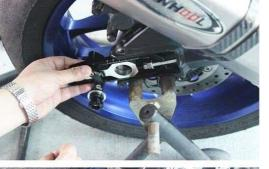
7. Install left & right side chain adjuster, tighten#2 original screws.
