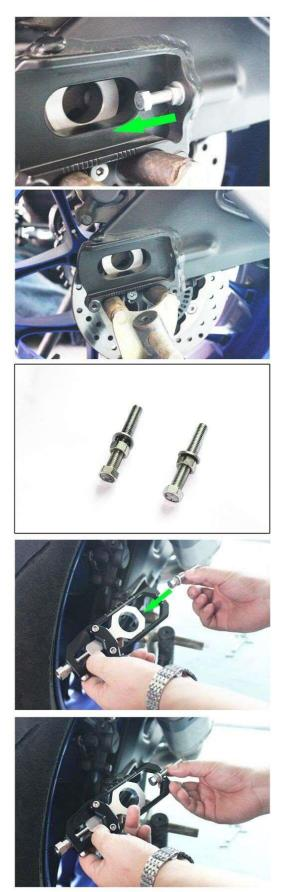
1. Remove rear axle lock nut & axle.
