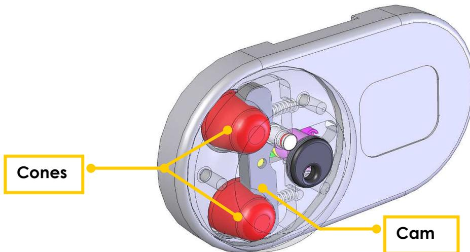
The double locking cone system ensures resistance and a space such as to allow the vehicle body twisting during traffic.
