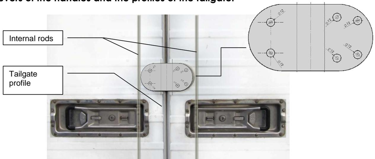
Pay attention to the edges of the door which can deform the drilling template sheet and then generate a misalignment of the holes.
