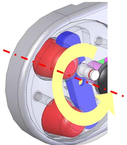
Similarly, burglary actions tend to remove the cam from its seat on one of the two cones are offset and inhibited by the other cone; act simultaneously on the two cones is not feasible or very complex.
