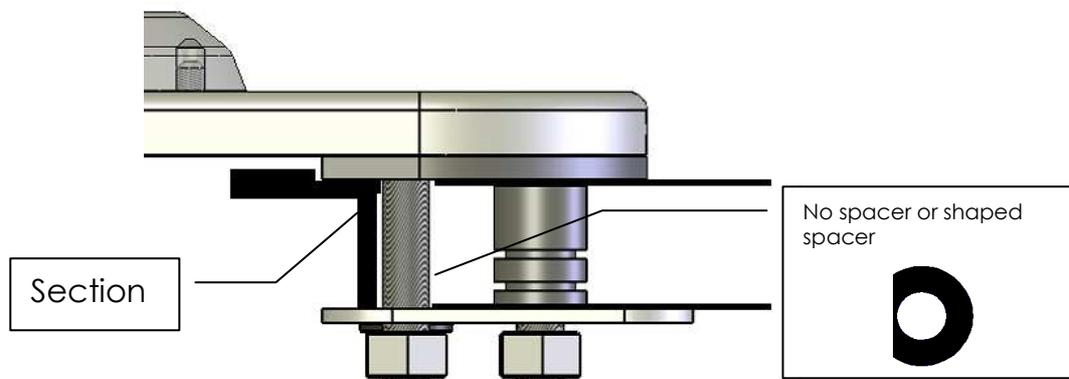
After making the counterbores from inside the door with a hole saw, wide the pre/hole with a tip of 11-12mm from outside the door.
