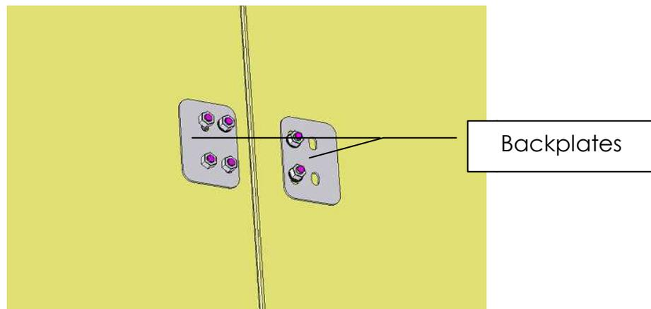
5. Before tightening the nuts verify the correct alignment of the lock with the locking cones. Perform repeated openings and closings with the lock opened. If necessary to contain any misalignments of the cones with respect to the body lock, apply one or two semicircular spacers supplied, placing them under the plate that supports the
