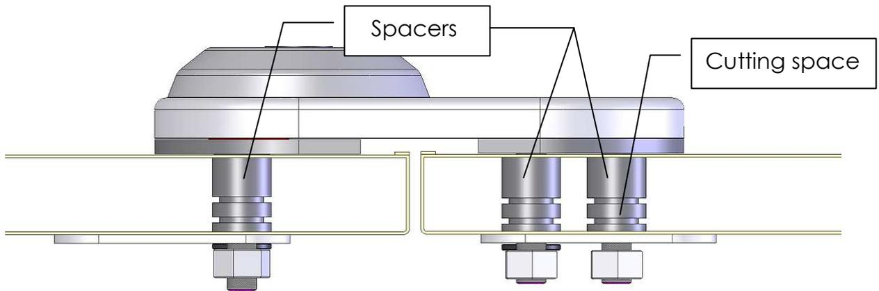
4. Finally, apply the inner backplates and the studs supplied. If necessary, shape the backplates (cut and bend) in order to avoid interferences able to deform the sheet metal.
