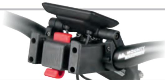
**Mounting** Enables use of the KLICKfix handlebar adapter in combination with Yamaha or Giant displays. Loosen and remove the lateral screws and attach the spacers with the enclosed longer screws.
