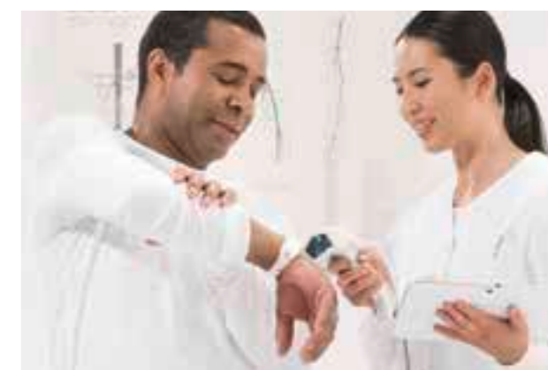
A standard bar code scanner can be connected via a USB port for use of the user and patient identification function.
