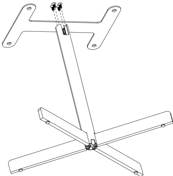
**5. Fix the top plate (B) to the tube (E) with the 4 screws (C)**
