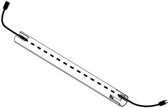
**3. insert the power cable through the tube (E)**
