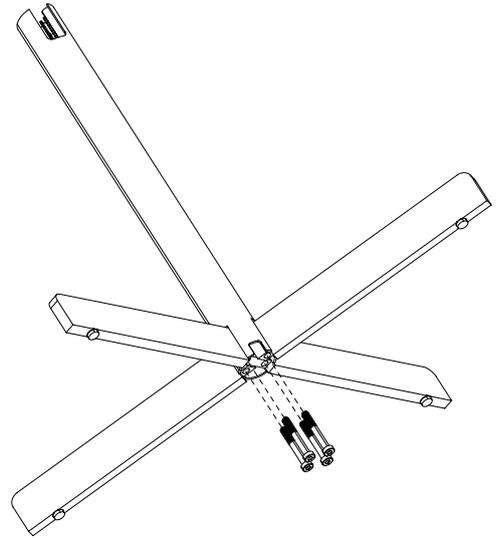
**4. Join legs and tube with 4 screws (L)**
