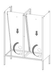
Push the back panels into place, starting at the bottom.
