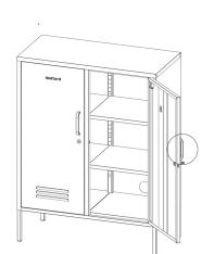
Use your screwdriver to attach the handles with the small screws + small washers.
