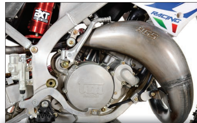
Left: HGS makes the exhaust for the stock models using a combination of a 125cc and 85cc system, while other aftermarket manufacturers like Bill's Pipes in the USA also
