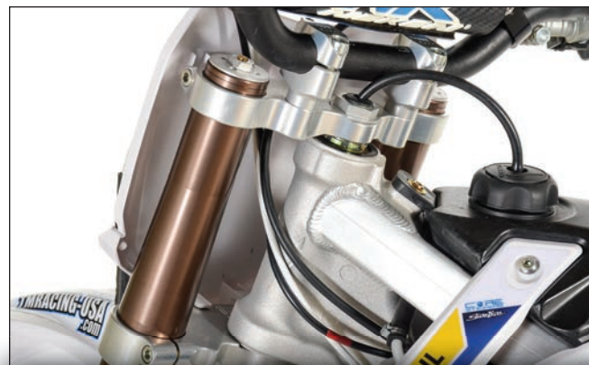
Left: Machined aluminum triple-clamp and bar mounts are stock items on the TM 112 Supermini. Right: To get the 112cc displacement, TM uses a 52mm bore
