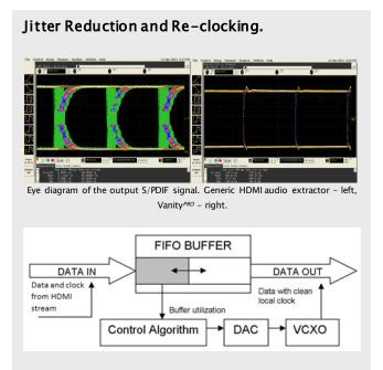
Audio data from the HDMI interface is buffered in FIFO memory and clocked out with local high precision oscillators. As a result, the output signal is completely isolated from the noisy HDMI domain – interferences from the power supplies, video circuits, etc.
