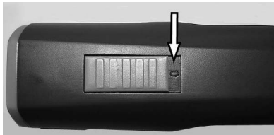
Fig. 4 Switch in OFF-position ("0")
