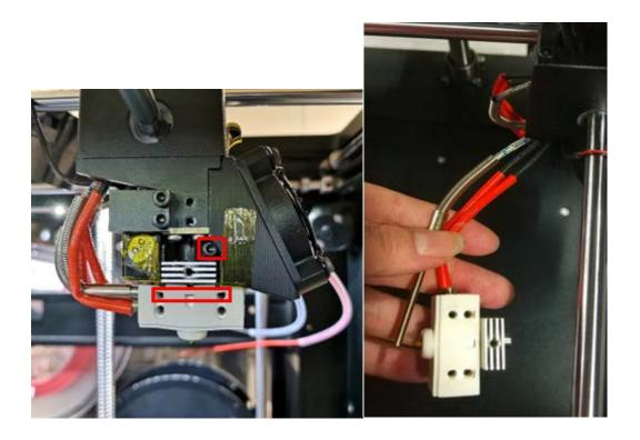
Remove Thermocoupler cable from extruder connection board with a flat head screw driver. Use a 2.5mm wrench to remove the two screws on the Extruder connecting board.
