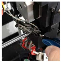
Pull the Thermocoupler wire out from the extruder carrier.
