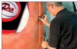
Warm up the film and roll RollePro simply over rivets channels, grooves or joints.
