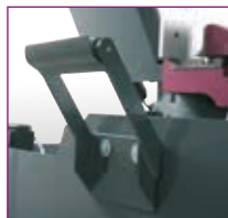
Roller support › For supporting long materials
