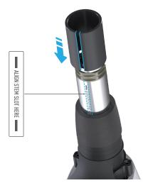
■ For non-Future Stems: Install a stem shim (S234800001) on the cartridge for all standard 1-1/8" stems. The shim slot needs to align with the mark on the Future Shock toward the back of the bicycle. You should be able to read the text through the shim slot.
