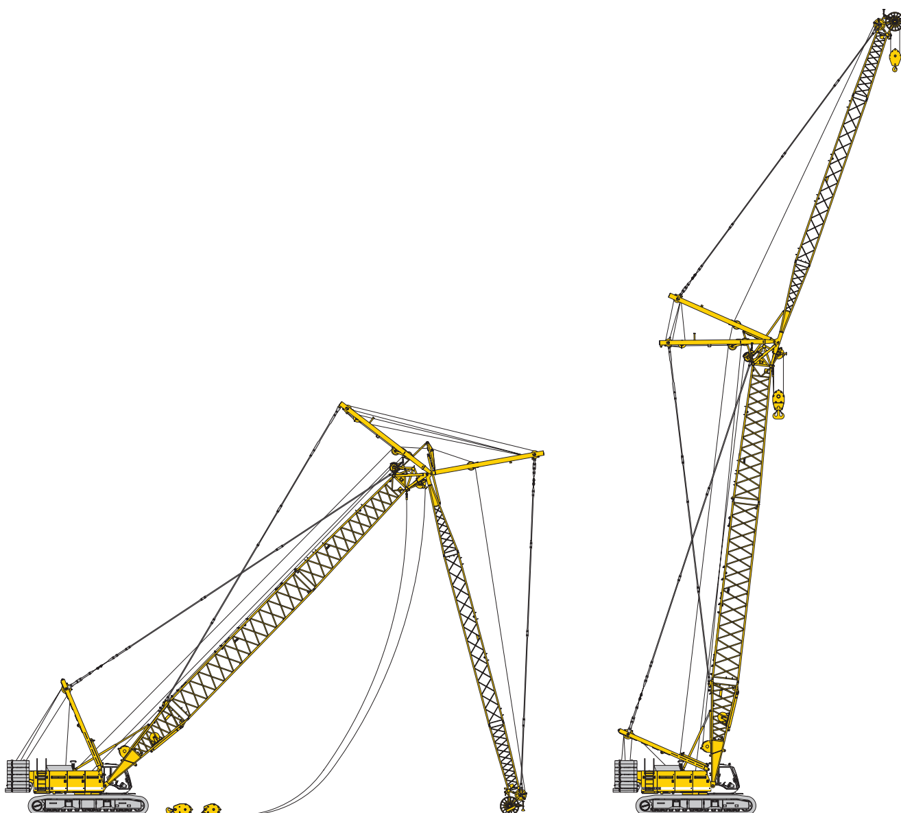
Erecting of main boom and luffing jib
