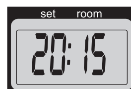
F: When the 4-digit stops blinking, the setting has been locked to the indicated value.
