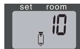
J: When the FUEL indicator has appeared, the information display will show the number of minutes of fuel left in the tank.
