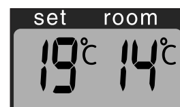
F: The required temperature on the left, the measured temperature on the right.
