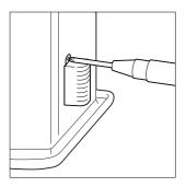
2. Remove the connector by holding with fingers and attach the extension wire.
