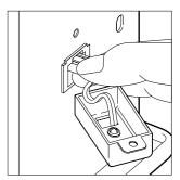
3. Attach the extension wire to the connector on the side of the room temperature sensor.
