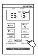
The childproof lock can be used to prevent children accidentally changing the heater settings. When the heater is burning and the childproof lock is on, the heater can only be switched off. Other functions are blocked then. If the heater has already been switched off, the childproof lock also prevents accidental ignition of the heater.
