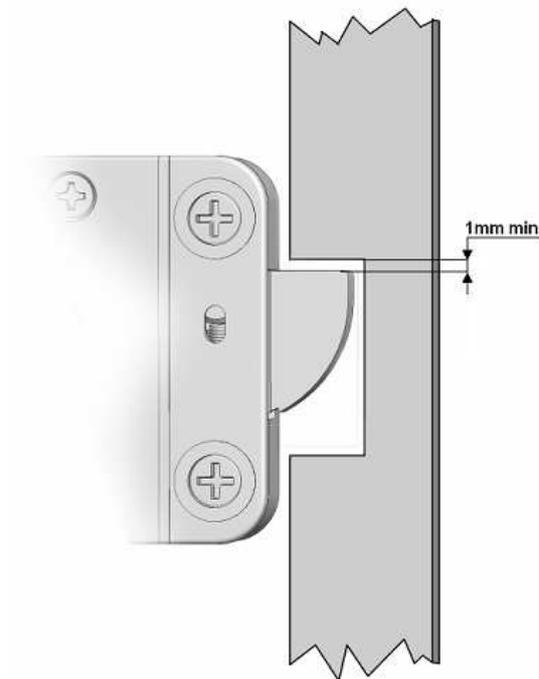
In the LOCKED position the distance between the DirectXion bolt and the boltwork part that is moving the lock bolt should be approximately 1 mm.
