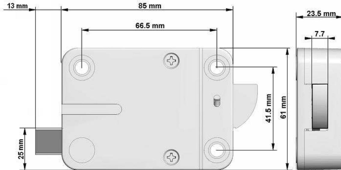
Connection to lock is via a RJ45 (female) connector on lock case. Cable (Art.nr. 390) has to be ordered separately. Min voltage: 9V, Maximum voltage: 12V.
