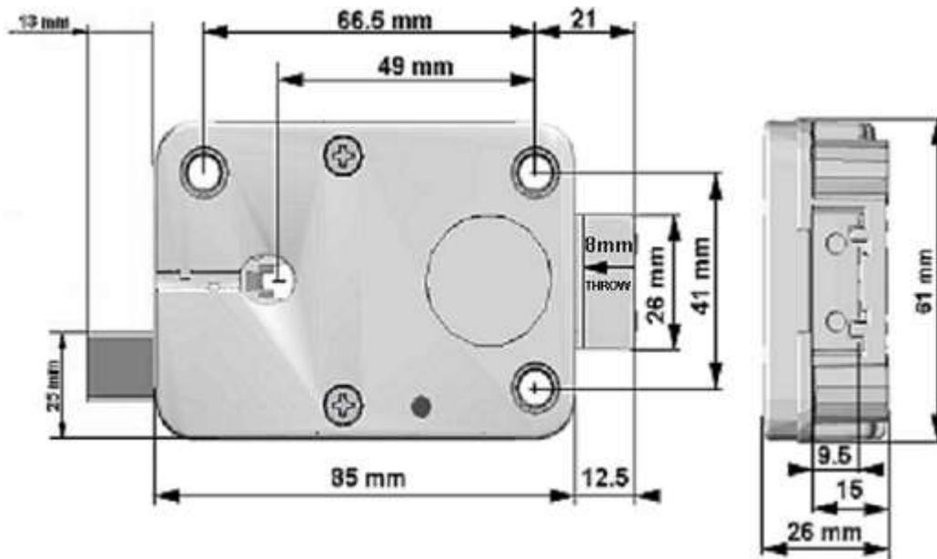
Connection to lock is via a RJ45 (female) connector on lock case. Cable (Art.nr. 390) has to be ordered separately. Min voltage: 9V, Maximum voltage: 12V.
