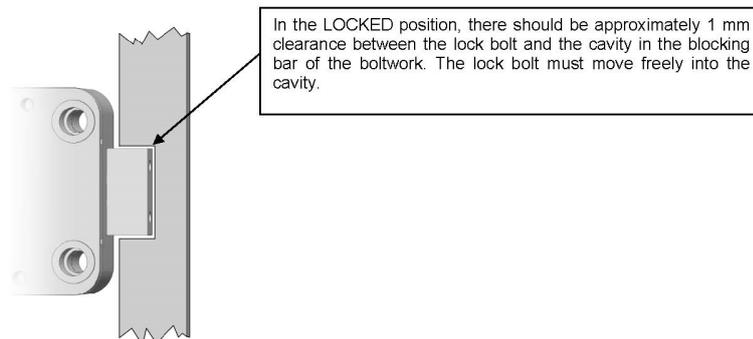
Only use supplied screws to mount the lock. Tighten the screws securely so the lock body is attached firmly to the mounting surface.
