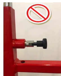
Fig. 4: Pin DOES NOT LOCK extension
