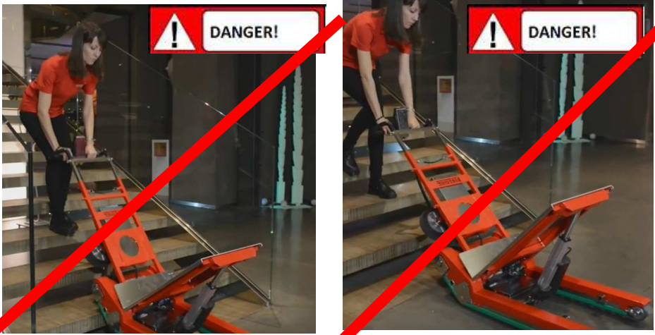
Figure 62: Mistake to be avoided: going down the flight of stairs without closing the load inclination.
