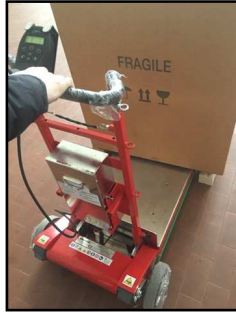
Figure 23 - Positioning the trolley under the load.
