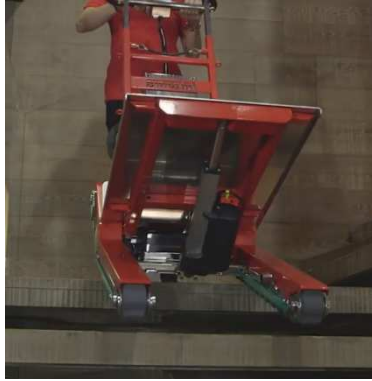
Figure 57: example of equilibrium position on the last step of the flight of stairs
