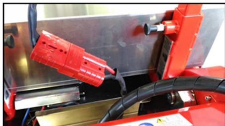
Figure 18 - DOMINO stair climbing trolley in transport configuration / Pins for locking the control handle.
