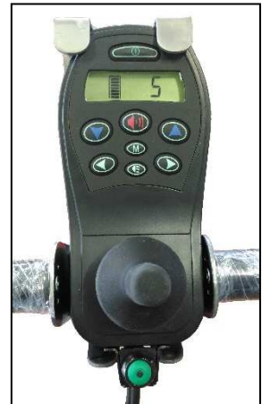
Figure 41: Display fitted on the control console of the DOMINO AUTOMATIC trolley.
