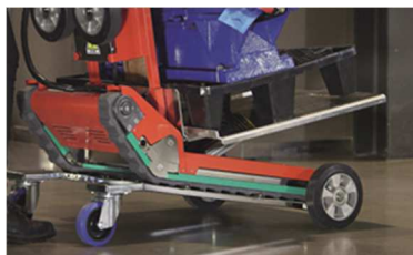
Figure 27 - Lifting the DOMINO stair climbing trolley onto the wheeled base.
