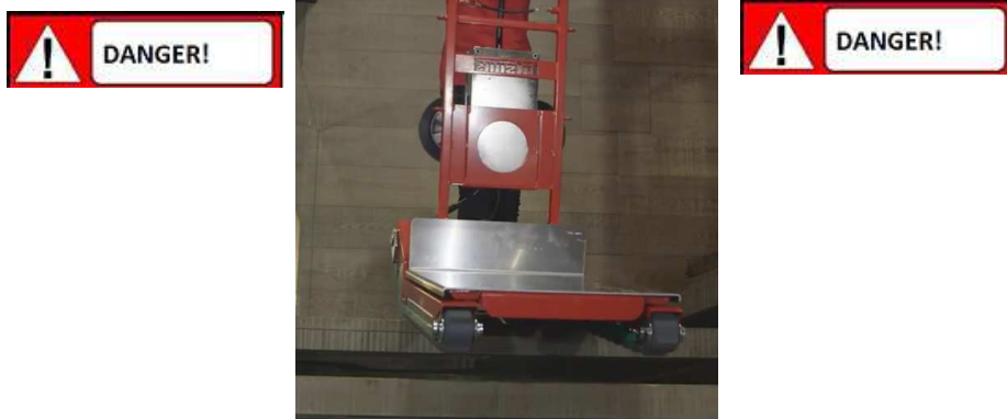
Figure 59: example of equilibrium position on the last step of the flight of stairs
