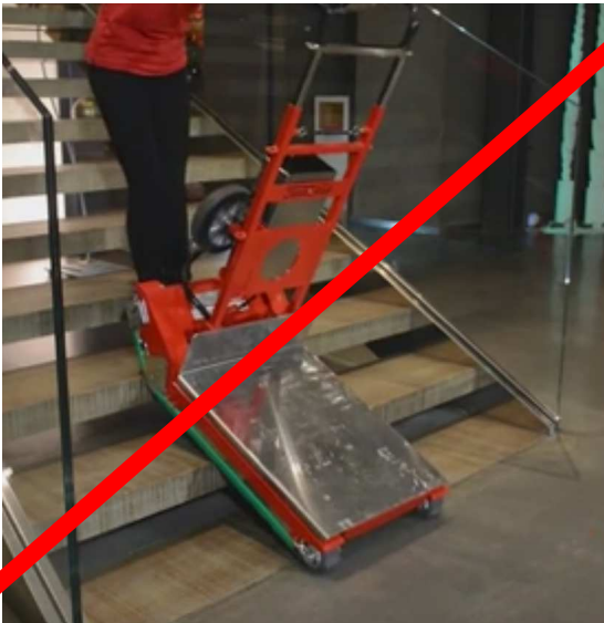
Figure 54: Mistake to be avoided: to start climbing the stairs without tilting the load
