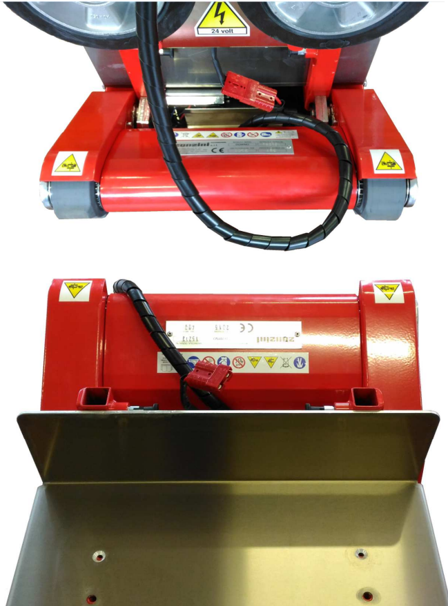
Figure 11 - Guards and protective devices of the DOMINO stairclimbing trolley.
