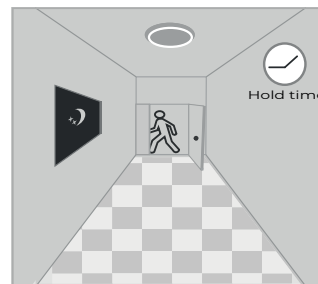
After the last detection and the present hold time elapsed, light OFF.
