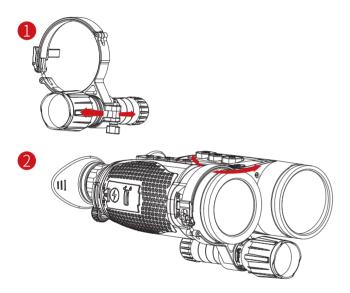
Figure 5 IR Illuminator Mounting Illustrations
