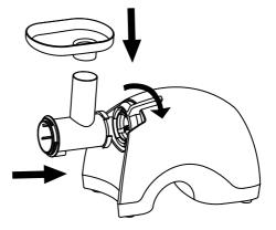
3. As shown in the picture, match the Twin Gear to the one point between the two points.
