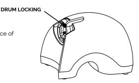
Assemble the feeding entrance and the drum, connect the drum to the main body, and then close the locking device by turning it to 'CLOSE'.
