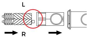
4. With the gear on the right, which has the axis of the Twin Gear, fix it to the drum together with your desired screen.
