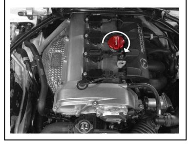
2 Continue tightening the oil filler cap until the "MX-5<sup>®</sup>" logo is positioned parallel to the SKYACTIV<sup>®</sup> logo as shown below. Finally, clean the oil filler cap with a clean soft cloth.
