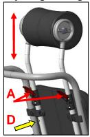
To adjust the height of the headrest, tip both levers (A) up and push the headrest to the appropriate height.
