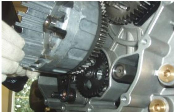
**Disassembling the clutch**
