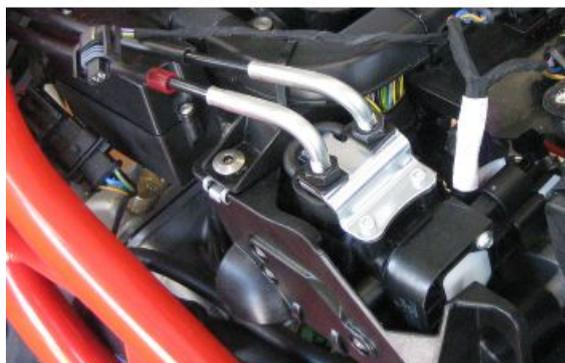
**Level in electrical circuit diagram:** Throttle grip position sensor.
