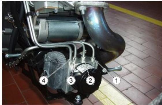
**Note: First of all, detach the brake pipes that go from the ABS control unit to the brake pump (1-4) and immediately seal the opened unions of the ABS control unit with protective caps. Afterwards, remove pipes (2-3) that go from the ABS control unit to the brakes and also seal these unions with protective caps.**
