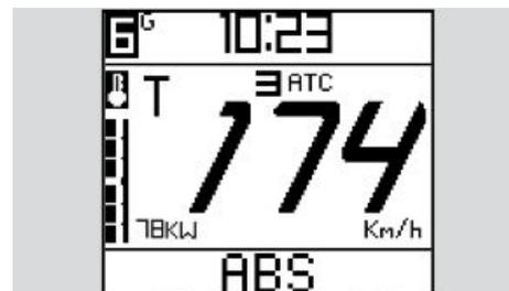
By moving the selector to the right - pressing it briefly - the ABS system turns on and the warning light starts blinking.
