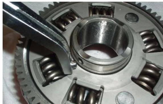
Check for any damage or signs of wear on the clutch bell that could lead to irregular clutch functionality. Grind down the teeth or replace the bell if necessary.
