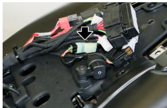
2. Signal - Pink/White colour, from VEHICLE PIN 65 to the fall sensor, passing through multiple connector - Section 0.5
