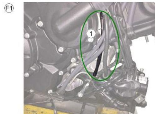
**TABLE G - PROCEDURE FITTING THE ABS CONTROL UNIT CONNECTOR CORRECTLY**
