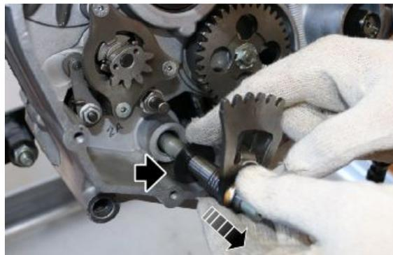
**Checking the gear selector**
