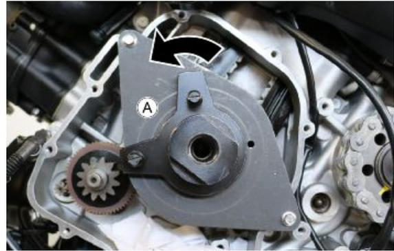
If necessary, remove the distribution gearwheels from the cam shafts:
