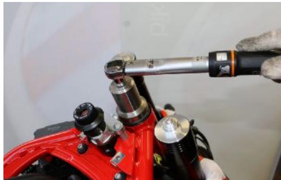
**Specific tooling****020884Y 46 mm wrench for steering ferrule**
