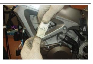
• Disconnect the alternator connector.
