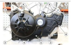
• Remove the clutch casing, retrieving the gasket, the two locator pins and the starter motor transmission gear.
