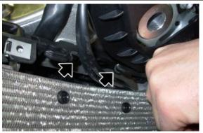
• Moving the bracket outwards, it is then possible to remove it by sliding it out.
