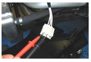
• Take the measurement; The correct value is determined by the value measured for each stage in which from time to time the resistance of the tester wires is subtracted, obtained by touching the two lugs.
