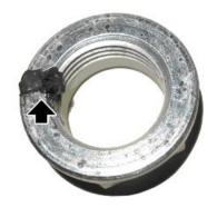
• Fit and the washer and the swingarm pin fixing nut on the pin and hand-tighten the nut.
