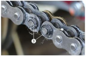
• Compress the outer plate (4) using the appropriate generic tool.
