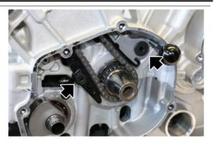
Unscrew and remove the two head fixing screws (a - b) from the flywheel side.
