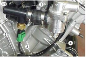
1. Injector 4 cable harness connector (output "6")
