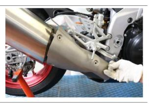
Loosen the clamp between the exhaust terminal and the central manifold.
