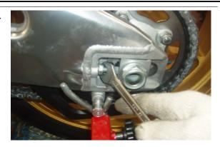
• Place the two washers and tighten the pinion fixing screw.
