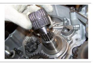
• Install the clutch gear, making it mesh with the oil/water pump control gear
