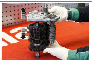
Remove the shim washer (5) that is located on the secondary shaft between the shaft and the cover
