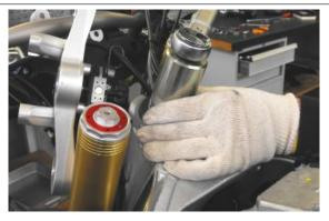
• Place the safety washer, bending two opposite tongues inside the ring nut notches.
