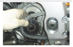
• Fit the pinion and the chain on the shaft.
