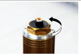
• Unscrew the upper cap from the sleeve using a specific Öhlins tool.
