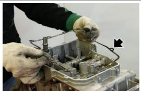
• Remove the overpressure valve together with gasket
