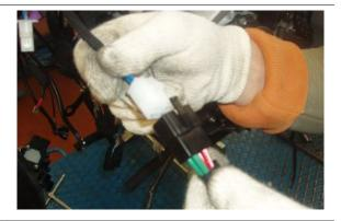
Connect the voltage regulator connector.
