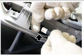
Remove the cable clamp fastening screw and release the shock absorber wiring harnesses
