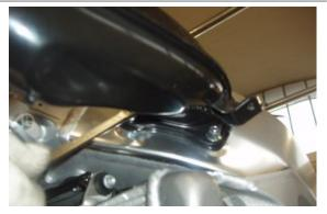
• Remove the duct from its seat on the frame.
