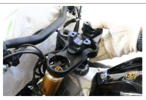
If necessary when removing the steering yoke, remove the wiring cable secured to the part positioned above it (where necessary).
