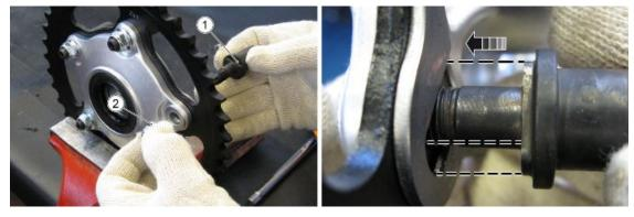
Block the rotation of the pins with a hex wrench (1) (EVEN IF THE FLANGE IT-SELF DOES NOT ALLOW THE RO-TATION) and tighten to the prescribed torque, the nuts (2) diametrically opposed in the order: (A) (B) (C) (D) (E).
