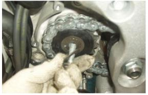
• Loosen the drive chain adjuster screws.
