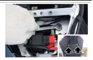
• Remove the cover placed under the tail fairing.
