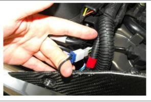
• Cut the ties fastening the cable harness to the engine.
