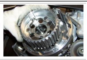
• Remove the clutch hub cam tower.
