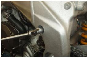
• Unscrew and remove the three plate fixing screws and remove the plate.
