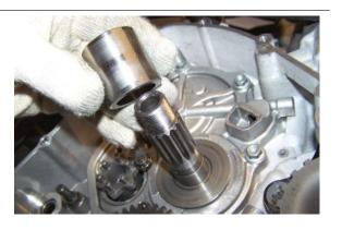
• Remove the thrust bearing.
