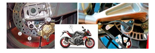
When sensors (3) detect a significant speed difference between the rear and the front wheels (for example, when rearing up on the back wheel), the ABS system could take this as a dangerous situation. In this case, 2 things may occur:
