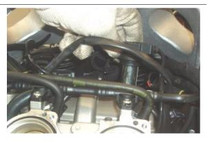
• Unscrew and remove the front spark plug.
