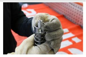
• Remove the pre-loading spring retaining ring.
