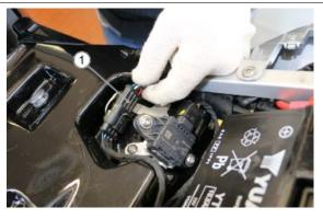
• Disconnect the connector (2) of the inertia platform.
