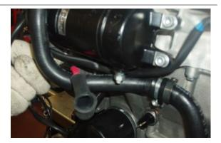
• Tighten the engine oil pressure sensor.
