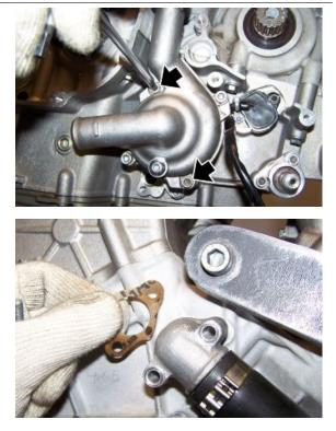
• Undo and remove the two fastening internal nuts of the water tank.
