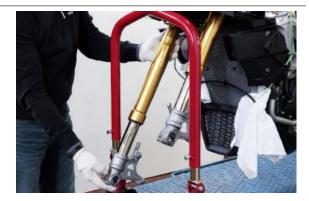
• When replacing the stanchions, take care when regulating the degree to which they protrude, following the instructions provided in the "Settings" paragraph in the "Suspensions" section.
