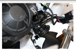
Remove the headlamp from the top fairing undoing the four fastener screws
