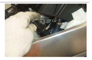
Remove the engine oil pressure sensor.
