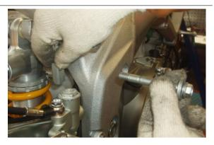
• Unscrew the upper adjuster screw bushing until it turns no more.
