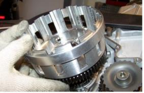
• Remove the clutch gear that controls the oil/water pumps
