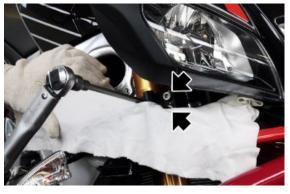
• While supporting the stanchion, loosen the screw on the upper yoke.
