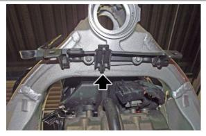
Use clamps to secure any axial movements of the hoses.
