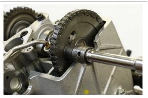
• Slide and remove the gear from the intake camshaft
