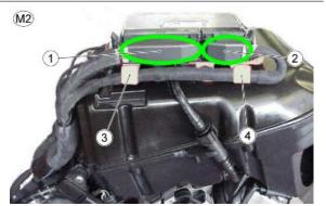
3. Cable harness routing (output "25") under the mounting
