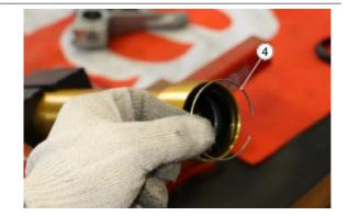
Remove the shaft seal (5) by levering
