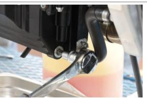
• Unscrew and remove the filler cap.
