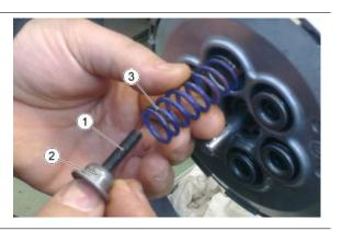
• Tighten the six screws operating in stages and diagonally.
