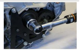
Insert the tone wheel on the crankshaft.
