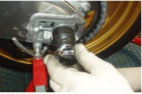
• Adjust the drive chain adjuster screws.
