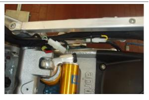
• Place the radiator frame, the washer and tighten the screw, fastening the frame to the engine.
