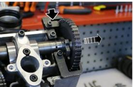
• Check that the camshaft gear works properly: if it is damaged or does not move smoothly, replace the timing chain and the camshaft gear.
