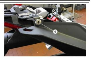
• Remove the rivet (5) placed in the lower part of the fairing.
