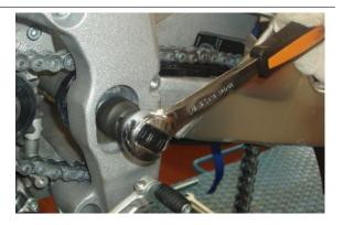
• Working from the right side, loosen and remove the locking ring nut.
