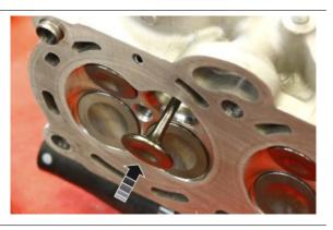
• Position the springs with the closest turns facing the head of the valve
