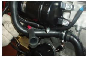
• Unscrew and remove the screw, remove the cable grommet and detach the three ground cables.
