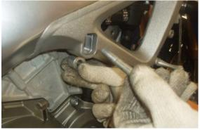
• Unscrew and remove the screw and retrieve the nut.
