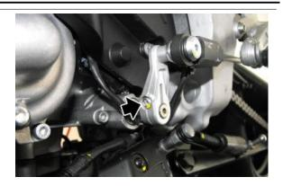
• Position the quick-shift cable harness and fasten using ties.
