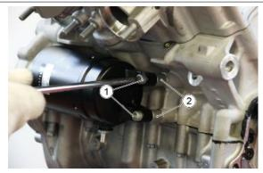
• Remove the starter motor (3) from its housing.
