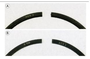
The five ring gaps (two piston rings, two oil scraper rings, one oil scraper spring) are fitted displaced 90° to each other, starting from the exhaust-side stud bolt opposite the chain and continuing clockwise.
