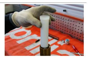
• Remove the wheel holder shaft (1) and the sleeve (2).
