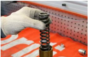
Position the ring-nut on the pre-loading spring and maintain it compressed while tightening the lock-nut on the pump
