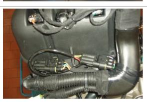
• Working from both sides, disconnect the Blow-by system intake pipes.
