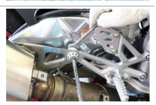
Rotate the exhaust terminal outwards slightly and remove the exhaust valve control cables.
