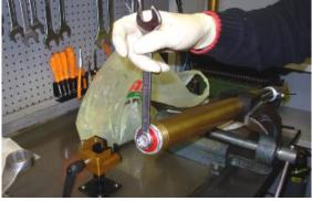
• Loosen the cover without unscrewing it completely.
