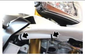
Remove the headlamp rim undoing the two screws
