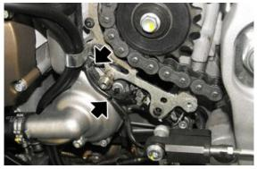
Loosen the screw and slide off the gear shift lever and cable harness from the engine.
