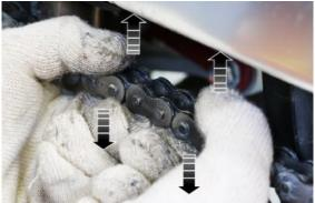
• Use a generic clincher to re-tighten the pins of the link (checking riveting at points "A").
