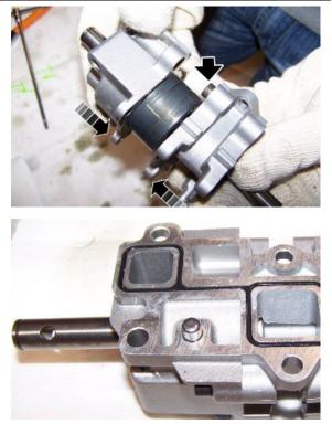
• Tighten the four lubrication oil pump cover screws.
