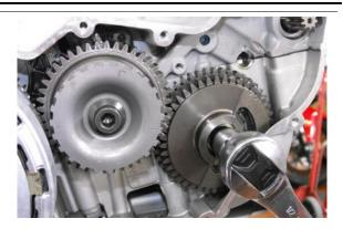
• Remove the countershaft from the alternator side.
