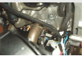
• Remove the front exhaust manifold.
