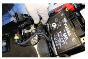
• Working on the left side, disconnect the tank's two vent pipes.
