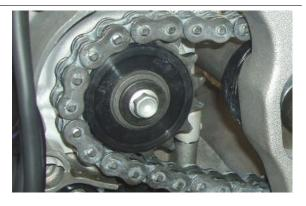
• Unscrew and remove the nut and retrieve the washer.
