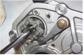
• Unscrew and remove the six screws.
