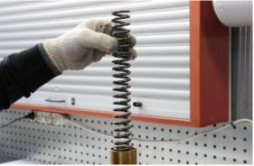
Position the ring-nut on the pre-loading spring and maintain it compressed while tightening the lock-nut on the pump
