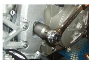
• Turn the swingarm pin (2) anticlockwise, which turns and loosens the adjustment bushing (3) completely.
