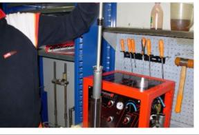
Using a hook spanner lock the pumping member pin and tighten the fixing screw on the fork end to the prescribed torque.
