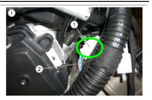
Gear sensor cable harness connector (output "15")
