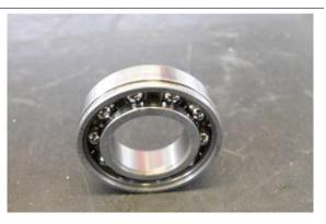
• Using the suitable tools, fit the bearing in the crankcase until tool stops.
