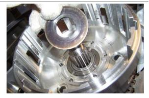
• Install the clutch hub cam tower.
