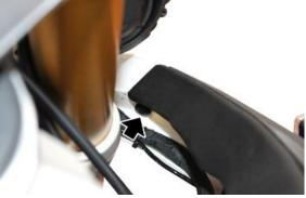
• Cut the plastic cable ties on the right of the top fairing.
