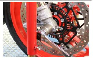
• Loosen the screws on the wheel axle clamps.
