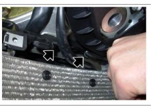
• Cut the clamp fastening the cable harness to the radiator return pipe on the left hand side.
