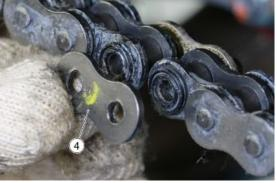
• Remove the outer O-ring rings (5).
