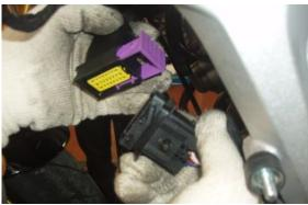
• Working on the right side of the vehicle, connect the exhaust valve control unit connector.
