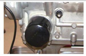
• Spread a thin layer of oil on the sealing ring of the new engine oil filter.
