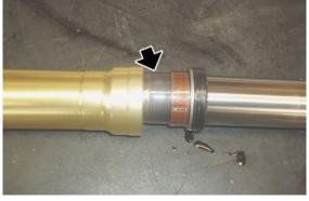
• Fit the sleeve on the stem and set the oil seal into position with the aid of the specific tool.
