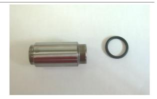
Compress the chain tensioner completely, making sure that the total length is 40.05 ± 0.5 mm (1.58 ± 0.02 in).
