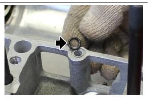
Insert the maximum pressure valve in the crankcase, composed of two separate parts
