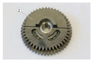
If deformations or broken material are found on the sliding surface, replace the freewheel gear (2). Check the freewheel sliding surface (2) for wear. Make sure that the woodruff key slot is in perfect condition.
