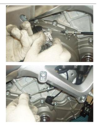
• Remove the timing sensor.
