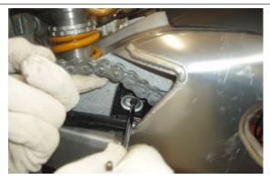
• Unscrew and remove the lower screw fixing the chain pad and retrieve the washers.
