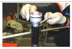
• Remove the spring pre-load pipe.
