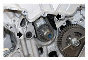
Unscrew and remove the two head fastener screws (a - b) from the clutch side.
