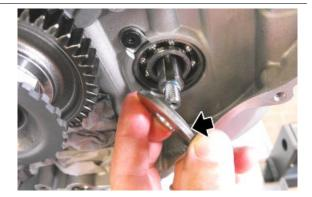
• Install the countershaft gear aligning the references on the countershaft
