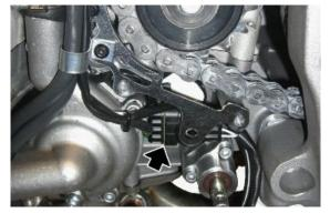
Unscrew and remove the screw from the cable grommet for the two exhaust butterfly valve control cables.
