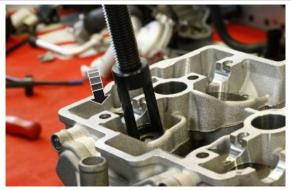
Release the wrench, checking that the ٠ cotters are positioned correctly in the valve grooves. ٠ Position the adjusting shims Position the bucket tappets. ٠
