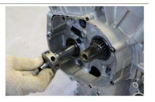
• Remove the countershaft gear.
