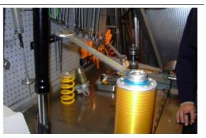
• Unscrew the upper cap from the sleeve using a specific Öhlins tool.
