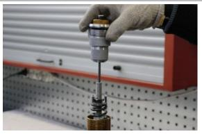
Unscrew the nut and remove it, exerting slight pressure on the pre-loading spring.
