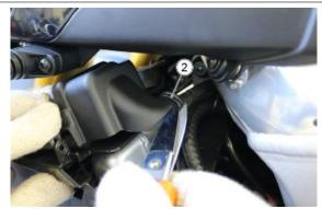
After detaching the ASC control unit (3) from the sub-fairing, complete with the cover (4), separate the two components.
