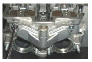
• Remove the cover together with the two secondary air system valves.
