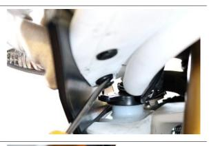
• Remove the front rivet on the bottom side of the inner top fairing.
