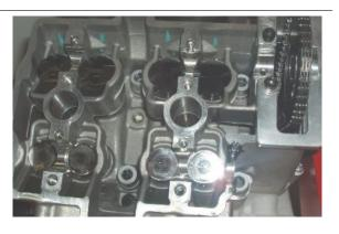
NOTE THIS ENGINE HAS CAMSHAFTS OF THE EXHAUST VALVES WITH CLEARANCE RECOVERY.
