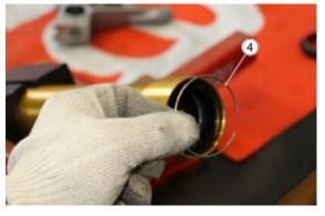
Remove the shaft seal (5) by levering it alternately at various points.
