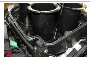
Working from both sides, unscrew and remove the air pressure sensor fixing screw.
