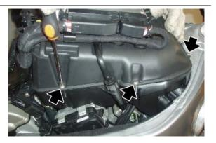
• Disconnect the upper injector fuel delivery union.
