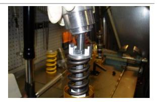
Unscrew the nut and remove it, exerting slight pressure on the pre-loading spring.
