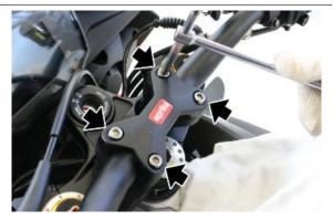
• Undo and remove the fastening cover of the upper yoke on the headstock.
