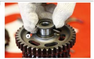
• Move the gearbox shafts together and fit them into the support
