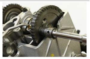
• Slide and remove the gear from the intake camshaft
