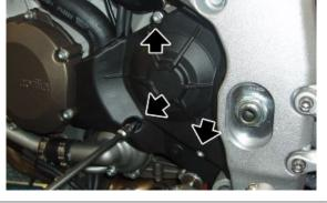
• Connect the vehicle cable harness / engine cable harness connector.
