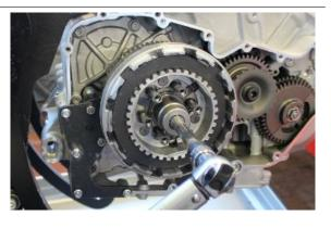
• Insert the disc with friction material and the black tooth into the bell.
