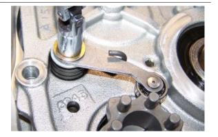
Check the selector shaft and its teeth for damage and wear.
