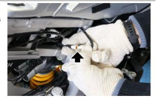
• Disconnect the compression electronic control connector.
