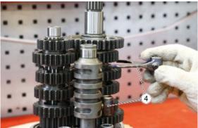
Remove both gearbox shafts from the cover
