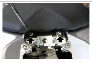
• Lift the rear saddle and slide it off the pin on the tank
