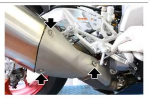
• Remove the heat guard making sure to recover the washers.
