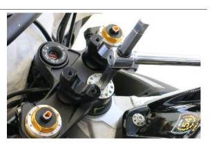
• Loosen the screws fixing the fork stanchions to the upper yoke.
