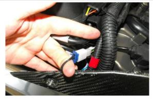
• Connect the alternator connector.
