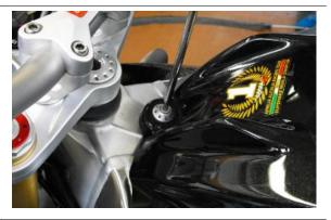
Unscrew and remove the two rear screws.
