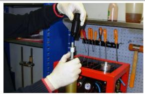
• Remove the lock nut and the washer.
