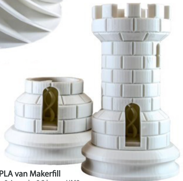
PLA Pro van Makerfill 120 mm/s, 0.4 nozzle, 0.2 layers, UM2+ Result after 17 hours
