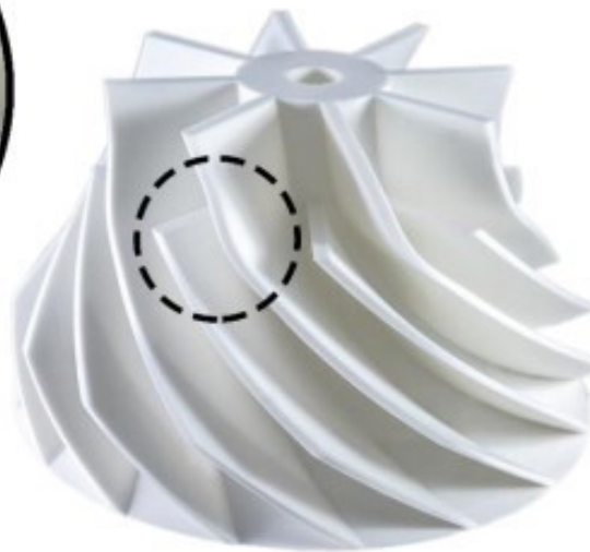
Close up of a printed object with PLA Pro (Printed on an Ultimaker 2+, 0.19 layer height, 242°C) Result after 17 hours
