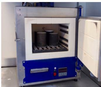
Place flasks in a well ventilated burnout oven.
