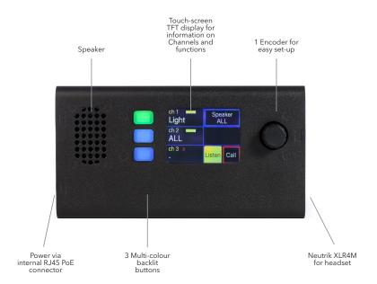
The Green-GO Wall Panel X Speaker version is a panel-mounted version of the Green-GO Beltpack with direct access to three communication Channels (either a single direct user or a group.) In addition there is a speaker with a separate engine to which any user or group can be assigned. For example program audio and stage manager announcements.
