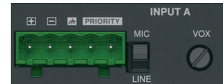
5-Pin Euroblock Connector - Remote
