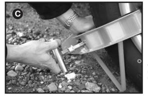
**C.** Once the optimum jaw position has been established, the jaws need to be closed by using the hex tool to turn the hinge bolt clockwise. Use the hex tool to achieve a secure fixing.
