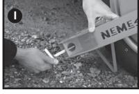
I. Once in position, tighten the Wheel Hub Arm Hex Bolt (7) by turning clockwise until sufficiently tight.
