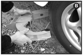
**NOTE:** The tips of the 'jaws' should be fitted into the wheel as far as possible. A little experimentation will be required to ensure a secure fit for your application.
