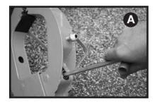
**A.** Using the hex tool (5), unscrew the hinge bolt (8) anti-clockwise to open the 'jaws' (1).
