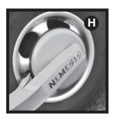
H. Hold the arm in position. The round wheel cover has a slide and tilt mechanism and should be adjusted to be central to the face of the wheel as much as possible. On larger wheels where central location is not possible. it must be ensured that at least one of the wheel nuts is covered.
