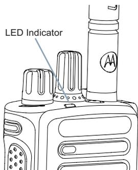
*The LED lights up solid green while the radio is transmitting and blinks when the radio is receiving.*
