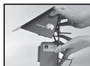
Place the cover with the solar panel back onto the base plate and slide the locking clip back into the 2 slots on the backside of the base plate.
