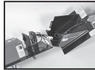
Remove the cover from the base plate. Take caution with the solar panel wires so that they remain connected to the base plate!
