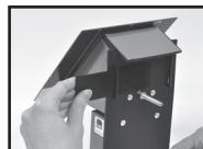
Remove the locking clip on the backside of the case by sliding it sideways.
