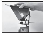
Carefully tip the cover with the solar panel forward from the underneath. Take caution with the solar panel wires.
