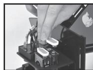
Insert 2 x 9 Volt block batteries into the battery compartment with the (snap) contacts facing upward. Connect both snap connectors to the batteries. Mind the Positive ⚡ and ⚡ Negative poles. (\*See chapter 1. Battery use)
