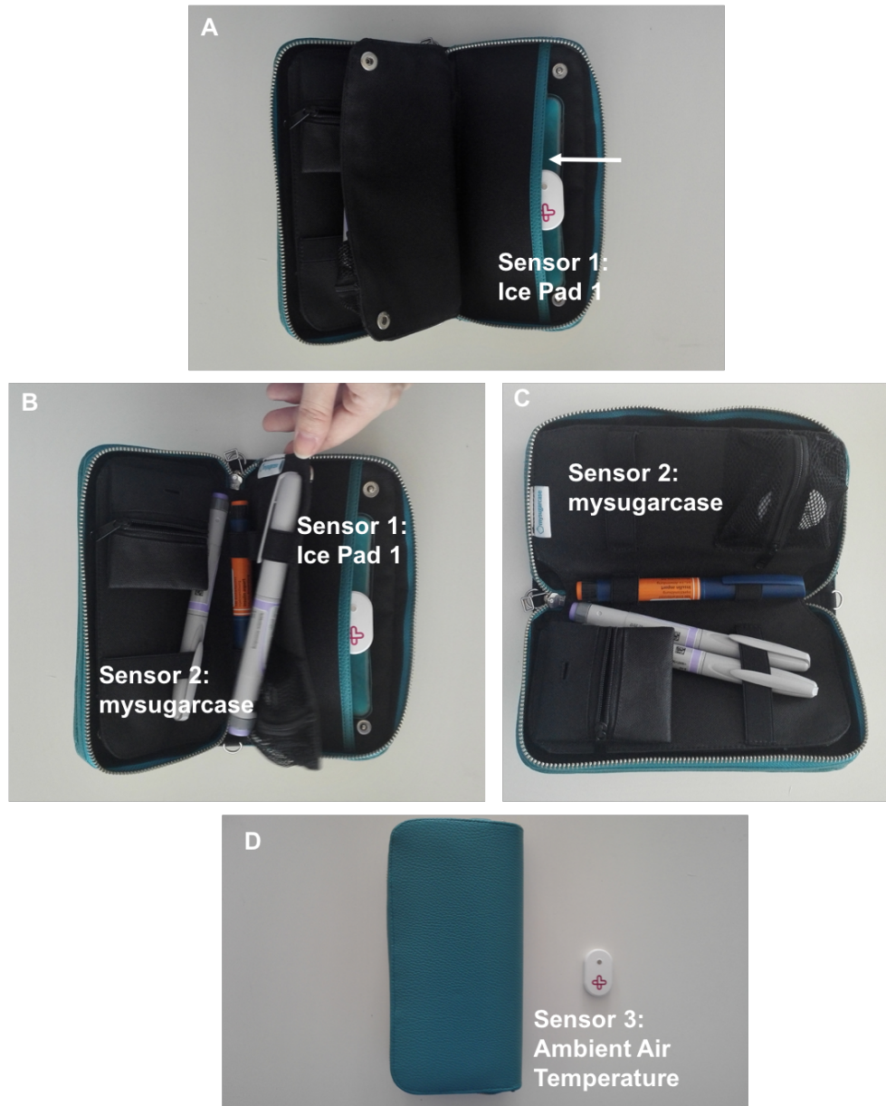
Figure 1: Test Arrangement. A) Sensor 1 ("Ice Pad 1") was put into the pocket with an ice pad, which had previously been stored in a freezer (-17 to -29°C) B+C) Sensor 2 ("mysugarcase") was placed in the mesh pocket of the inlay, next to the ice pad pocket (see B), also 3 insulin pens were put into the case D) Sensor 3 ("Ambient Air Temperature") was placed 10 cm next to the closed case
