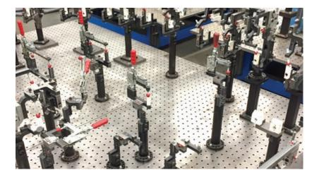
at a fraction of the cost. The fixtures could be printed and then used the next day on the welding table - and with minimized setup time, as each fixture is customized for its specific application. This provided a favorable contrast to using modular welding fixtures, which are imprecise and require additional time for adjustments to fit exact needs.
