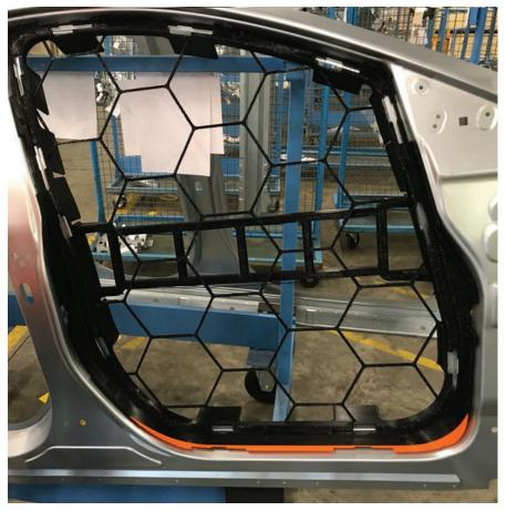
Traditionally-made hand jigs require many iterations and an 8-10 week lead time. By 3D printing them in-house iterations can be sped up and jigs can be created in just 2-3 days - a 94% time savings when comparing the new 3-day process to the traditional 50-day period.
