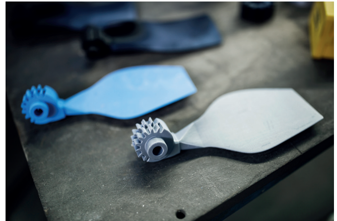
PLA propeller prototypes used by Sylatech for investment casting metal
