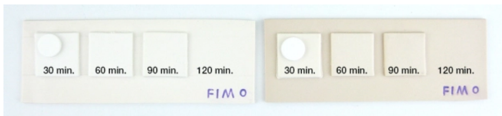
Squares are baked clay. Circles on top are raw clay. The left strip was double-baked. The right strip was baked normally.
