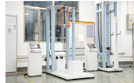
Frame vertical test
