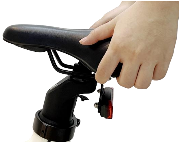
Step ①, loosen the seat pipe clamp.
