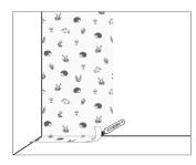
Adjust the length to the bottom of the wall and trim the excess wallpaper by using a ruler and a cutter.
